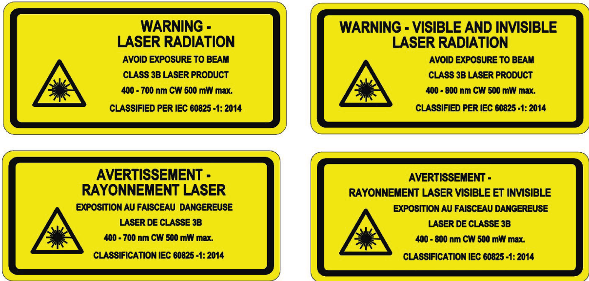
Figure 1: Versatile Laser Engine Class 3B Labels.
