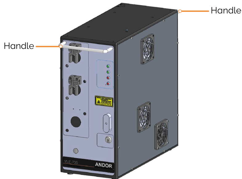
Figure 7: Versatile Laser Engine handle positions on front and rear of unit highlighted.
