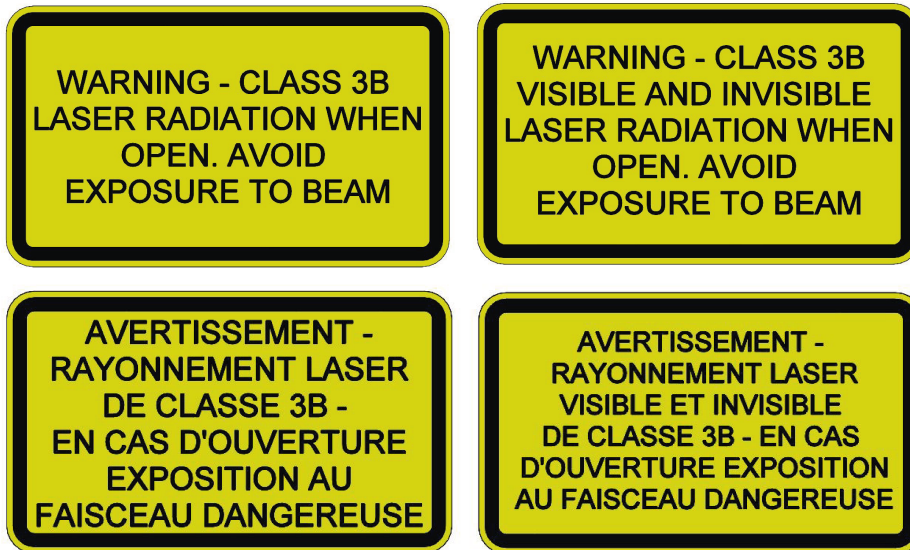
Figure 4: Access panel labels.
