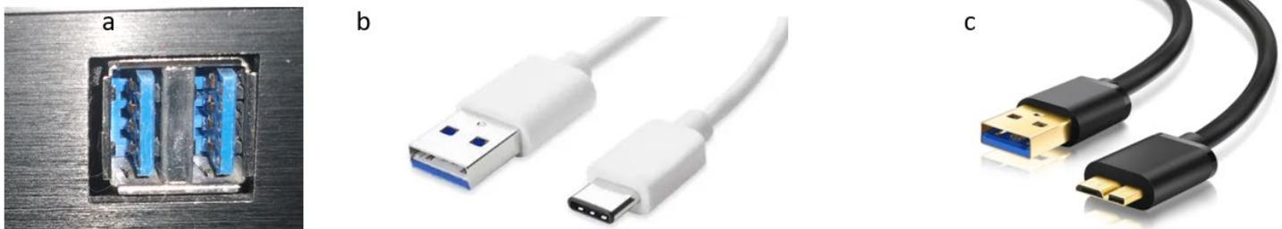
Figure 1 : Ports and cables used for USB connection of First Light Imaging cameras
