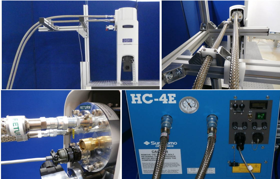
Figure 4-24: Connections between the GM compressor and cold head
