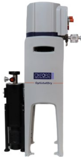
Figure 4-22: OptistatDry TLEX system after the removal of shipping fixtures
