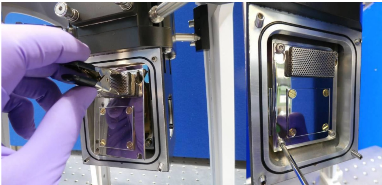
Figure 6.3: Replacing the sample access plate
