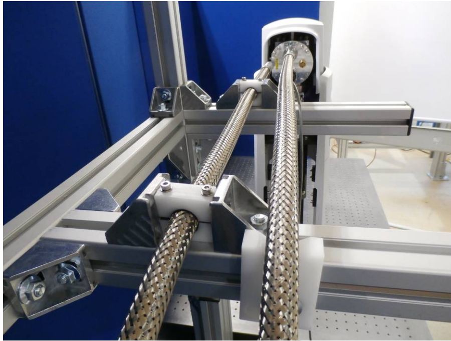
Figure 5.25: Support, but do not restrain, the return line
