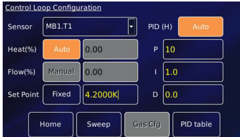
Figure 5-2: MercuryiTC 'Control' screen.
