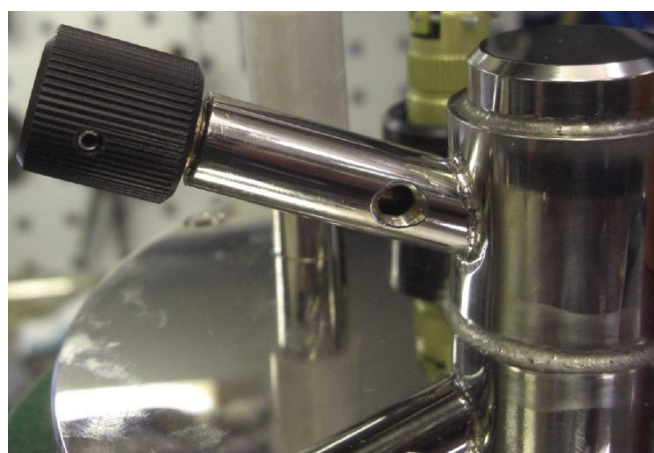
Figure 5-1: Optistat DN-V exhaust needle valve.
