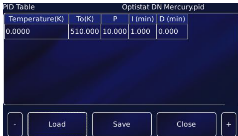
Figure 5-3: MercuryiTC Optistat DN PID table screen.
