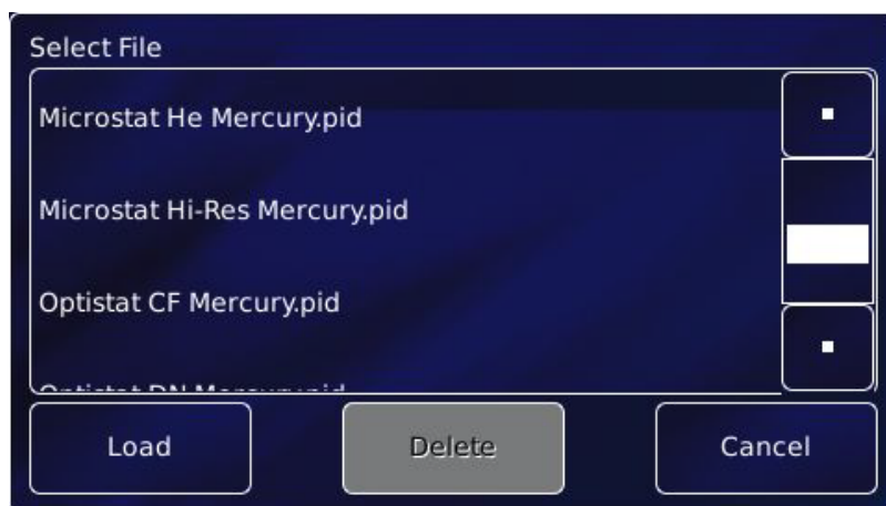
Figure 5-4: MercuryiTC 'select file' screen for loading alternative PID tables.
