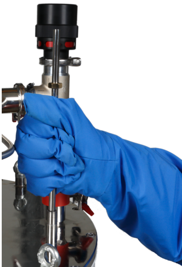
Fig. 3.8: Checking for nitrogen vessel blockages using a metal probe.
