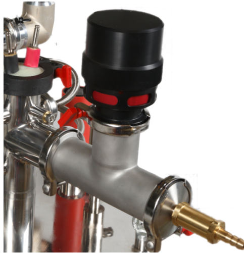
Fig. 3.6: Quench relief valve and non-return valve fitted to the helium reservoir exhaust of an Oxford Instruments cryostat.
