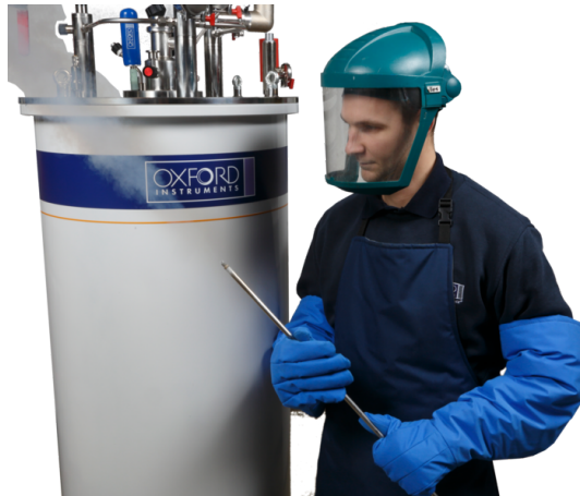
Fig. 3.1: A full set of PPE including cryogenic apron and gloves and face shield. The operator is protected from cold helium gas by gloves and face shield.
