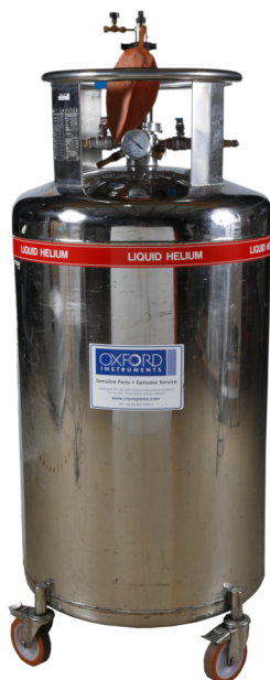
Fig. 3.4: A typical liquid helium storage vessel.
