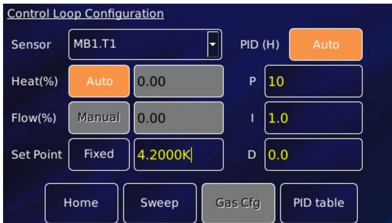
Figure 6.2: Mercury control screen
