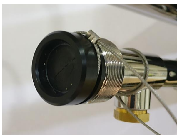
Figure 5-6: Special slotted bung fitted in the cryostat siphon arm.
