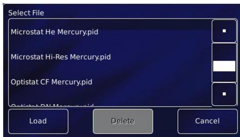
Figure 5-5: MercuryiTC 'select file' screen for loading alternative PID tables.
