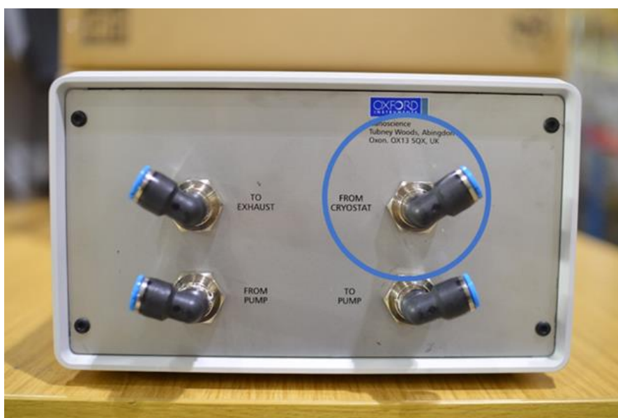
Figure 4-1: Rear view of the VC-U gas flow controller showing the connectors.
