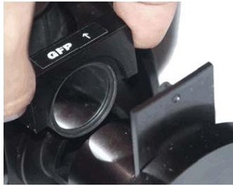
Figure 25: Inserting Excitation Filter
