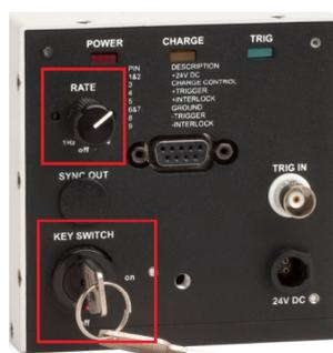
Figure 33: Set Trigger Rate - top left
