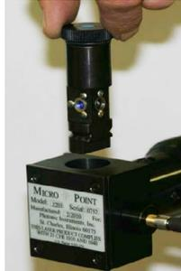
Figure 22: Removing/Replacing the Dye Cell
