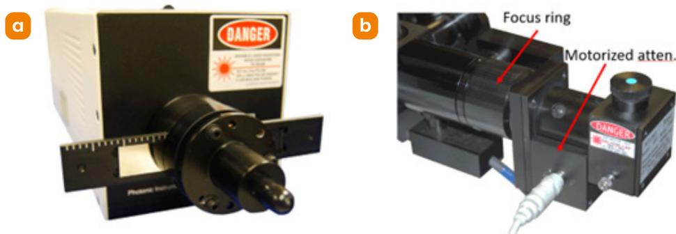
Figure 34: a) Manual attenuator slider on NL100 laser b) Motorised attenuator (0 - 3 OD)
