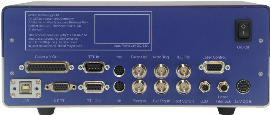
Figure 19: Connection Panel on MicroPoint 4 Controller
