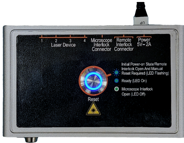
Figure 3: Laser lock box top panel view with solid blue LED indicating Ready (LED on).
