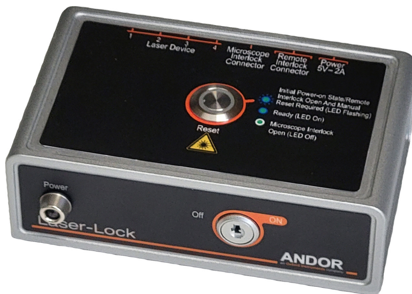
Figure 1: Front of the Laser-Lock Box, has the power LED and the key switch.
