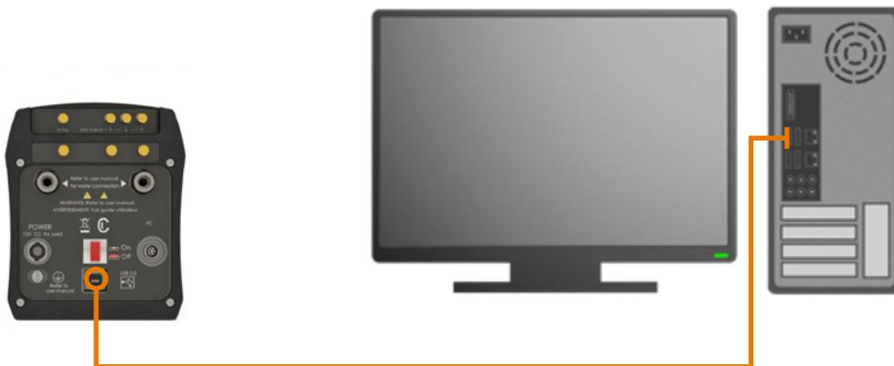
USB connection between camera and PC
