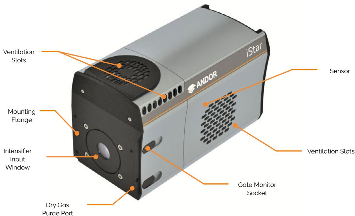
Figure 2: External features of the iStar CCD Camera
