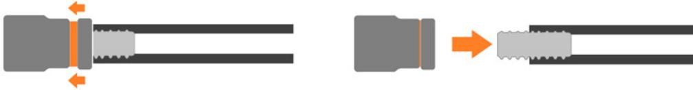
3. The hose should release from the camera connection with little resistance.
