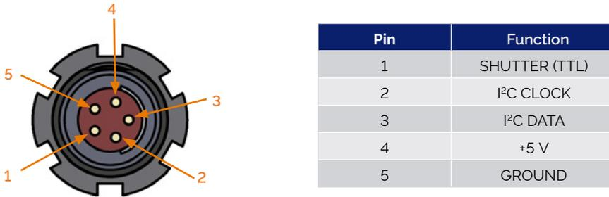
Figure 4: Pin outs of the I<sup>2</sup>C connector
