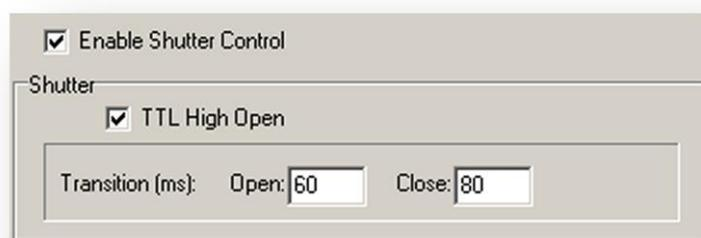
The Open/Close Transition time is the specified time the shutter will take to open or close. This time is used to give the shutter enough time to close before background data are acquired. The system ensures that a period of at least the duration of the Transition Time elapses between the shutter output signal entering the 'closed' state and commencement of background data acquisition.
