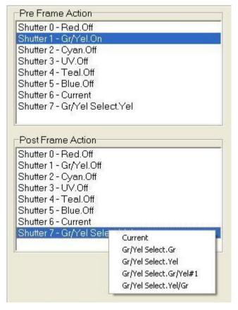
sure that the other TTL outputs are set to OFF (as shown) to ensure that only the Gr/Yel Source is ON during the frame acquisition.
