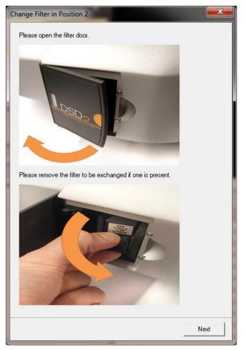
The DSD2 utilizes 4 individual filter cubes, these are changed using an access door on the side of the unit. Again the filters can be changed with the unit in situ. The filter change wizard will guide you through the process.
