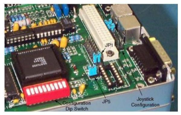
For instance, if the selected range is 1-10, and position 7 on the ten position jumper is selected, the module is set for address 7. Whereas if the selected range is 11-20
