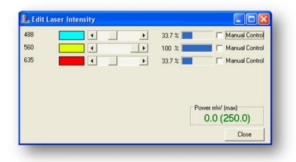
Each slider will change the intensity of the laser by adjusting the AOTF. The **Manual Control** checkbox allows the user to override the Channel settings and control the laser intensity manually during a Protocol. This allows on-the-fly intensity adjustments while executing a Protocol or use of a laser that is not in the Channels
