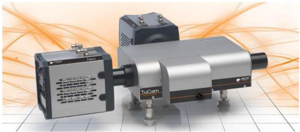
Andor has developed a flexible optical solution to split information between two cameras. The dual port camera adaptor (TuCam) shown allows dual wavelength or polarization imaging depending on which optical components are included in its modular optical cassette system.
