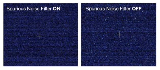
The above image demonstrates the effect of the Spurious Noise Filter on a dark image, 20 ms exposure, 200 MHz readout speed.
