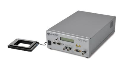
The Andor PZT-X00 Z stage can be supplied in ranges 100, 200, 250 and 500 nm. The 250 and 500 stages are required for multi-well or micro plate operation, having a large aperture to accept wellplate holder accessories.
