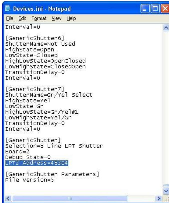
6. Now you have installed the Parallel port card and assigned its address, iQ will be able to write whatever digital patterns you wish to assign to the TTL outputs of the device.
