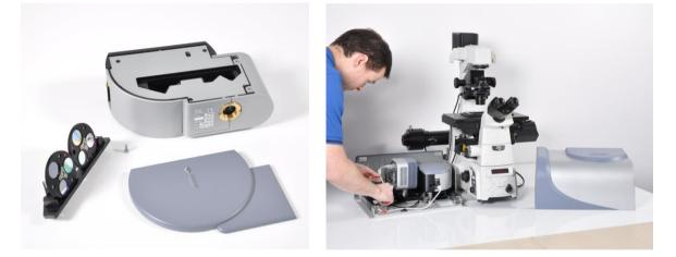
User access to DSD turret changes is especially convenient in the Andor design, and can be performed while the DSD remains attached to the microscope as shown. DSD2 is a newer variant of the DSD unit.
