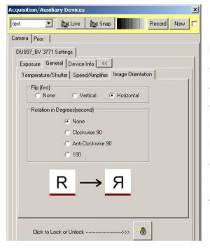
If you are using a camera which contains a back-illuminated chip e.g. iXon 897BV or 888BV, then you may have to flip the chip about the horizontal or vertical axis to correctly align the stage axes to the microscope. The chip is reversed in the housing to present the back of the CCD chip for illumination. Thus when the camera is readout one of the axes is reversed or flipped. Make sure you do NOT enable FLZ for Stage Alignment.
