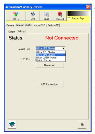
The LPT parallel port has 8 TTL output lines for control of hardware including shutters and other hardware such as Lumencor light engine, perfusion control and so on. The LPT1 interface is standard on Andor Imaging workstations (e.g. Dell T3500) but has been phased out by some manufacturers. Fortunately, you can readily obtain PCI and PCIe to Parallel port (IEEE-1284) interface cards at a very low cost. Examples below have been tested at Andor and showed robust behavior.
