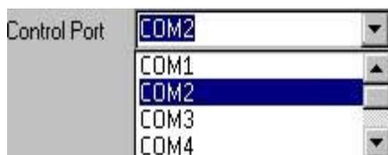
The filter wheel is controlled through one of the serial ports on your computer. From the **Control Port** dropdown select the port you are using.
