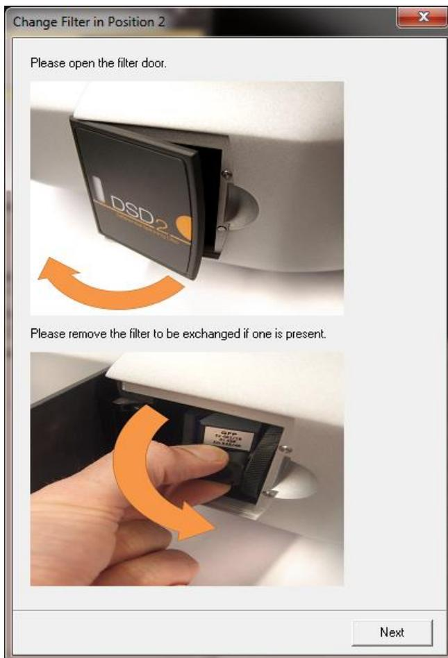
The DSD2 utilizes 4 individual filter cubes, these are changed using an access door on the side of the unit. Again the filters can be changed with the unit in situ. The filter change wizard will guide you through the process.
