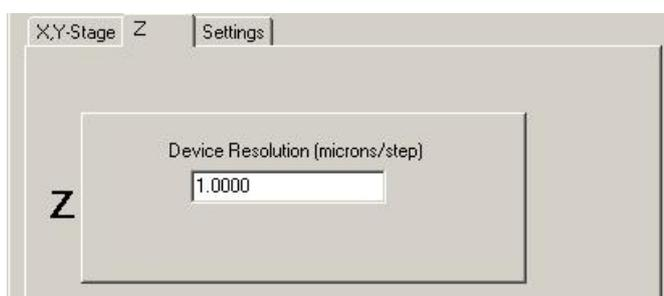
closed loop the motors are commonly set to 50 nm per step or 0.05 micron per step. Closed loop operation uses with a linear encoder gauge to monitor relative position of the stage and objective The linear encoder is attached to the microscope objective turret with a special bracket and the encoder reference plate is attached to a fixed plane on the instrument.
