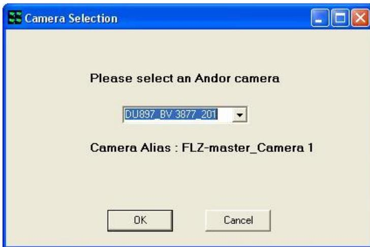
The camera selected using the drop down list and is identified by serial number – which is printed on the camera body for physical identification – in this case the SN is printed as X3877. Note is associated with configuration FLZ-master, which we created in the previous
