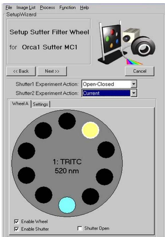
Various devices have shutters e.g. filter wheels, ALC, CSU. The state of the shutters must ensure that the desired imaging path is “open” for illumination and detection. To minimize specimen exposure and the side effects of photo-bleaching select the Open-Close Option for the fastest shutter in the path.
