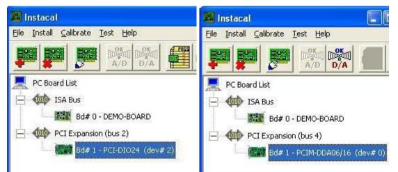
The above picture shows the card installed as Bd #1 in the Instacal initialisation program. Exit InstaCal.
