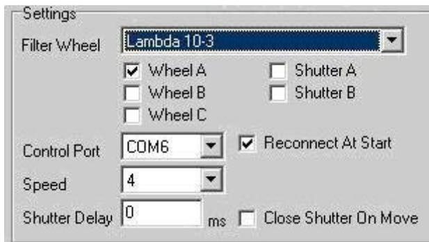
When you select one of the filter wheel options, the interface will provide a set of check boxes to tell iQ what you want to control, as shown left. Check the boxes of components you want to control.
