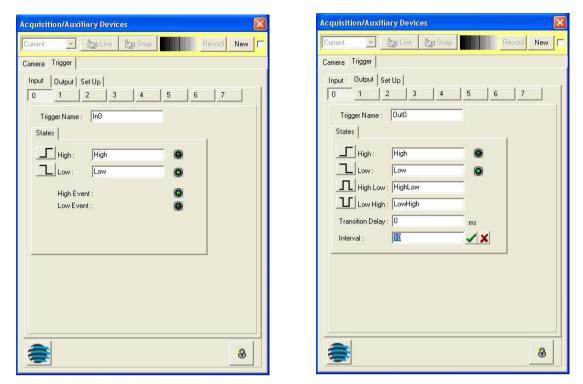
5. Depending on which TTL signals you intend to use, 0 thru 7 for Input and Output, you can monitor or set their status on these tabs. The 8 buttons along the top of each tab switch the user interface to reflect the current state of the relevant inputs and outputs.
