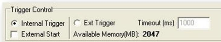
In addition, when two cameras are operated in synchronous mode, for example with the Andor TuCam, the first camera will be set to “Internal Trigger” and its “Fire” pin connected to the second camera’s “Ext Trig” pin. The second camera is set to “External Trigger” mode and thus the two cameras capture frames at the same moment.
