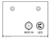
In order to control it for bright field imaging with FLZ you connect a selected TTL line on the PCU to the MOD IN input shown to the left. Note the LED illuminator connects to the LED connector.
