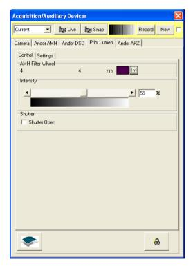
While the slider (the continuous grey-scale annotation) allows control of the output intensity setting with 1% increments (shown at 55% here). The device Shutter checkbox switches the continuous shutter between the slider setting and zero output.
