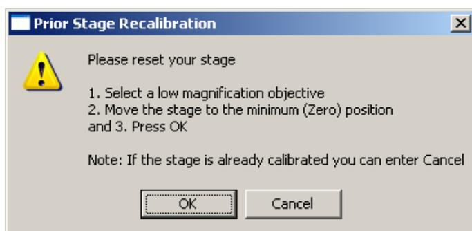
the recognised stage position has been lost and the device needs to be reset.
