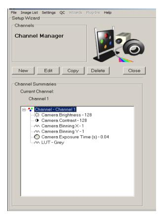
complex acquisition sequences (Protocols). Channels specify settings for cameras, microscopes, filter wheels and shutters – in short anything affecting sample illumination and image capture.
