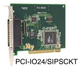
The card delivers 24 TTL signals, but we make use of 8 inputs and 8 outputs.
