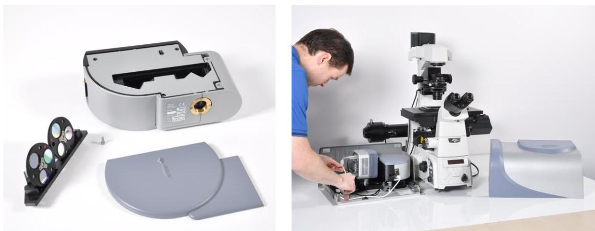
User access to DSD turret changes is especially convenient in the Andor design, and can be performed while the DSD remains attached to the microscope as shown.
