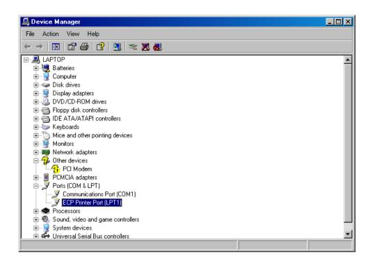
The Parallel port should appear as ECP or EPP in Device Manager. If it does not appear, or is listed as SPP, restart the PC and change the parallel port settings in the BIOS. If you are not happy with this step, contact IT support or a computer-competent person.
