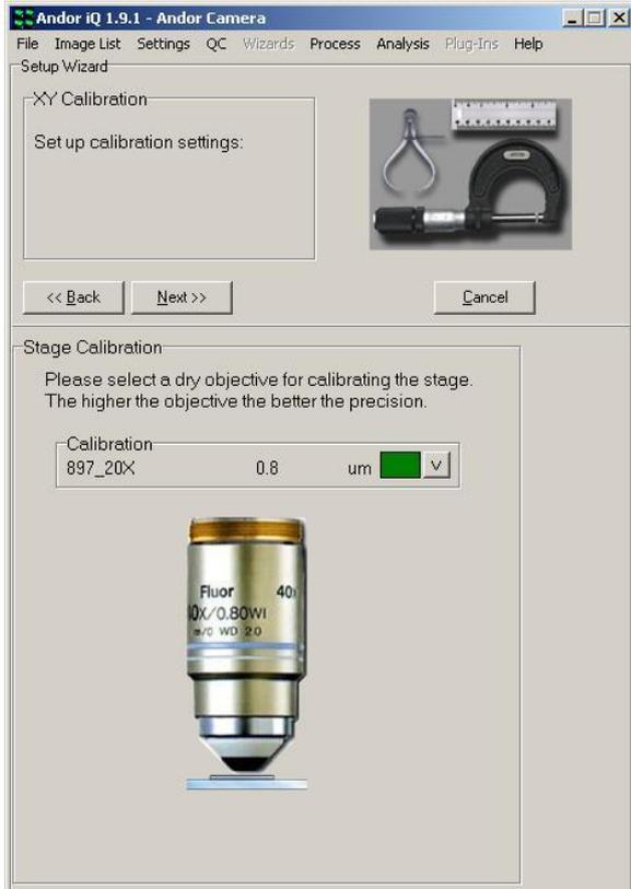
As this process proceeds you will be asked to rotate the camera or the stage. On an inverted microscope the latter is not possible, so the camera may need to be adjusted. So be prepared!
