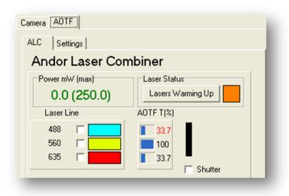
of the Protocol. Enabling Manual Control will change the colour of the intensity in the main AOTF window to red to show that it is no longer under control of the Channel. This is shown here for the 488 laser.
