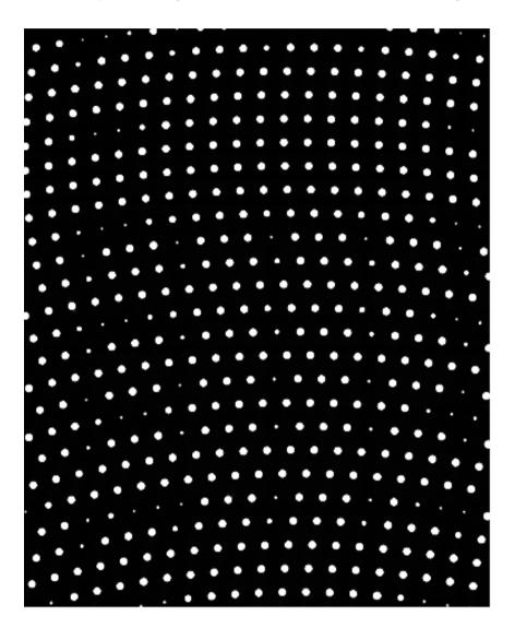
The dimmer circles correspond to areas where the grid lies. Please make sure that the grid is aligned properly (see following image for example) and that no circle is fully hidden. Once the image is acquired, please continue reading the "Calibration Process" section below.
