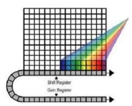
Cropped sensor mode is ideally suited to a number of challenging applications across manv diverse fields of research. The fundamental advantage and a distinct feature of EMCCD technology is its ability to virtually eliminate the camera readout noise detection limit at any readout speed. This allows EMCCD detectors to be successfully used for
