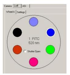
A common configuration is to use one wheel for Excitation and another for Emission, or you can configure a dual excitation wheel configuration in which one Excitation wheel contains ND filters for intensity control and matching between channels. If two or three filter wheels are selected Wheels A, B and C will show individual tabs on the Ludl Interface.
