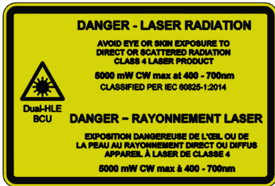
Figure 2: Dual-High Power Laser Engine BCU Class 4 Labels, location on the top of the BCU. These labels are not provided for a BCU driven by a single HLE as the label on the HLE is sufficient to cover it. However, in a dual-HLE configuration the output of the BCU is a combination of HLE outputs and so the combined power must be given.
