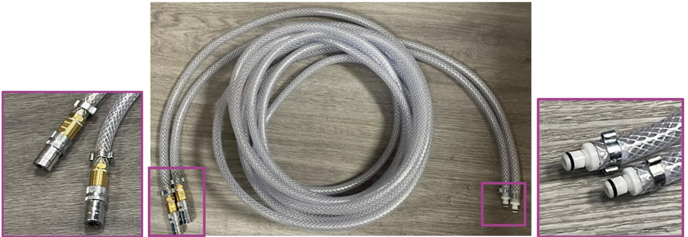
Figure 7: Water pipes with the hydraulic connectors for the cooling plate (left side) and for the chiller (right side)
