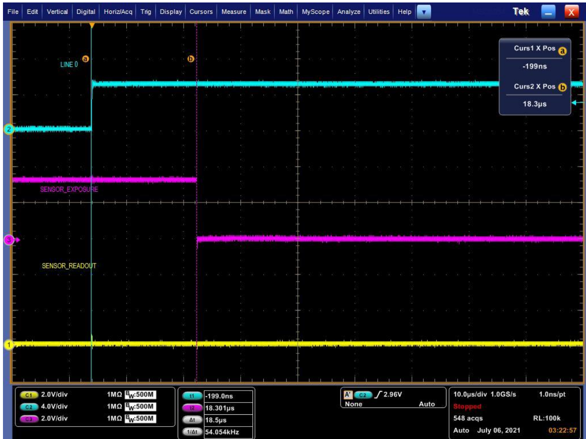
Figure 30: Example of the 12bits post exposition delay, here 18.30 μs
