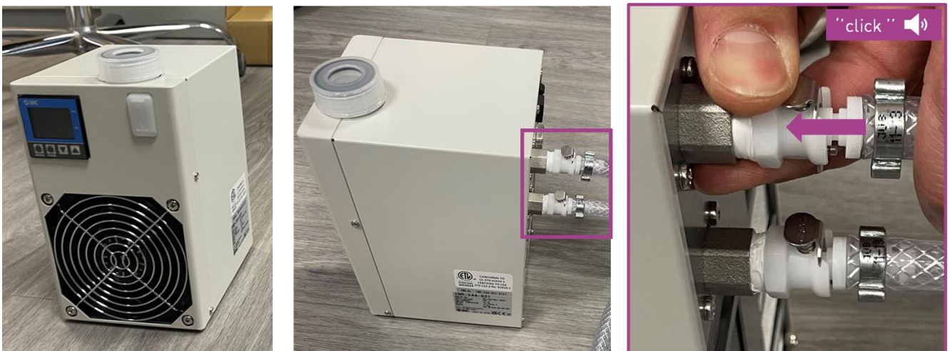
Figure 8: Cooling system main block. Left: front view. Center: side view. Left: pipe connection
