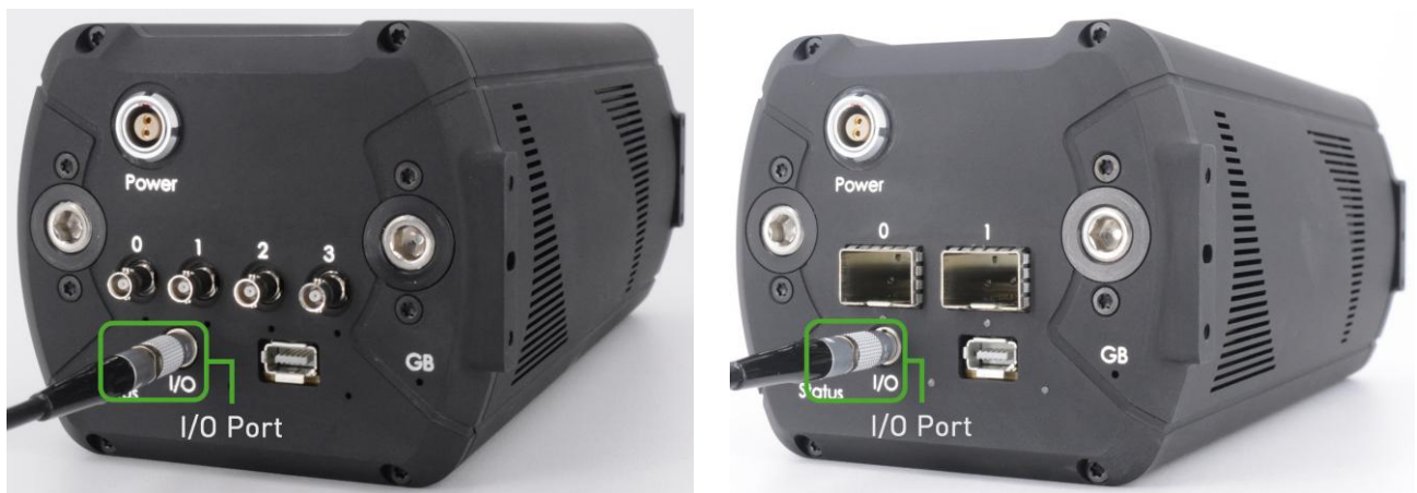
Figure 13: Andor CB2 I/O LEMO Port. Andor CB2 CXP is on the left, Andor CB2 SFP is on the right.
