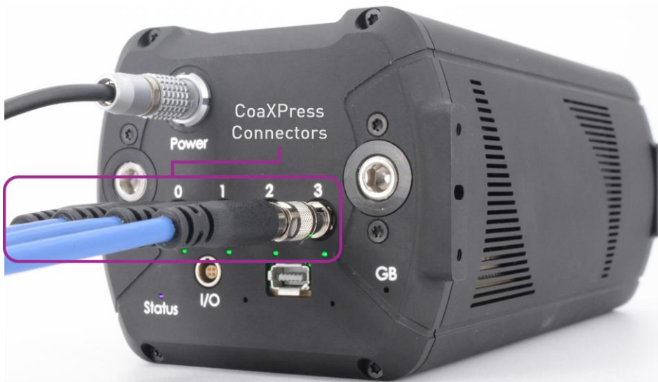
Figure 16: Andor CB2 CXP back view. The HD-BNC connectors are plugged in.
