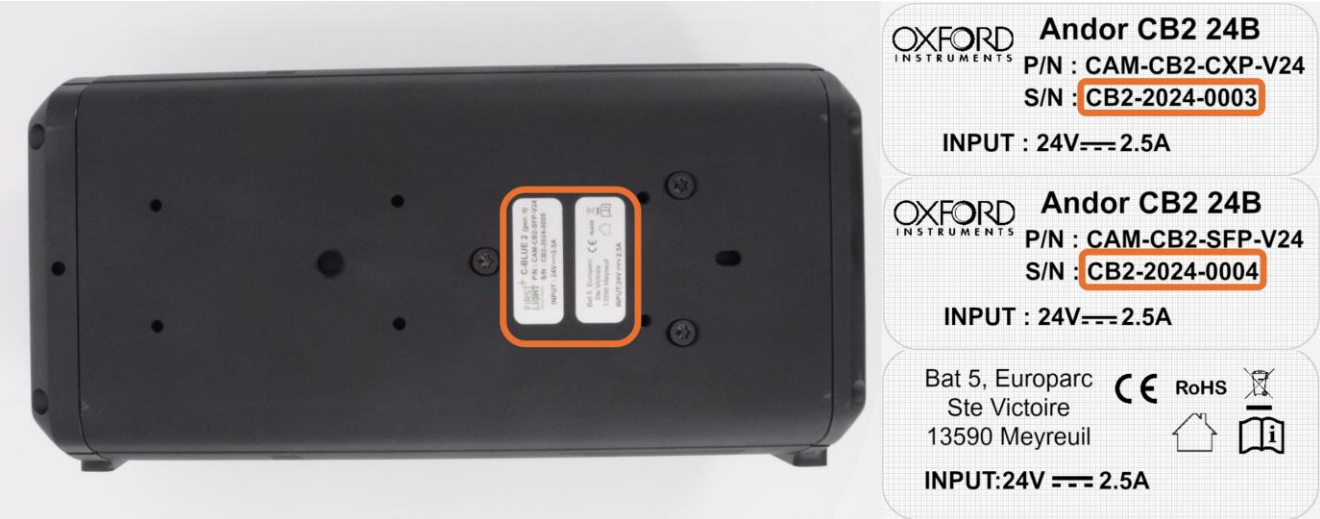
Figure 3: Stickers at the bottom of the camera, with Serial number (S/N) indicated.
