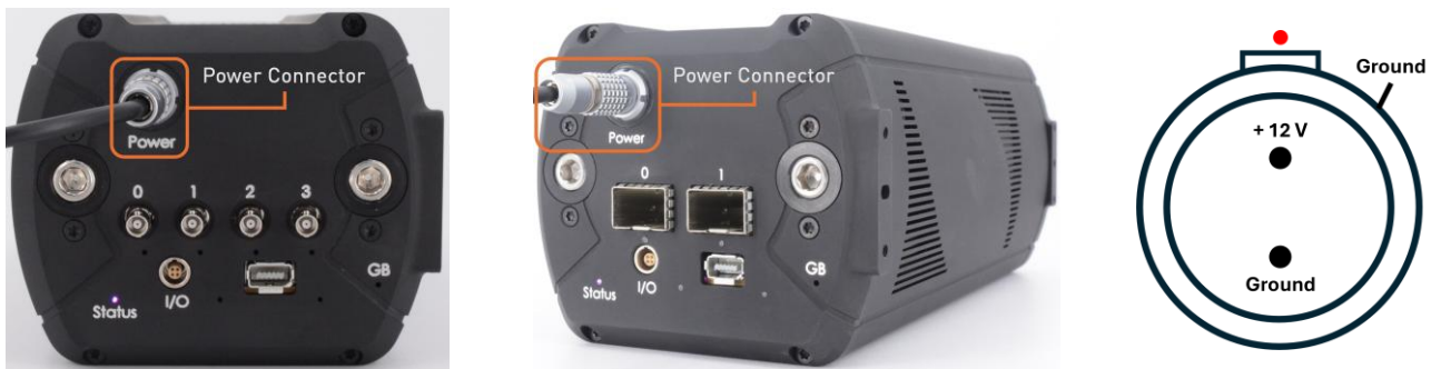
Figure 11: On the left, Andor CB2 CXP back views. The orange box shows the female power connector. On the center, Andor CB2 GigE Vision back views. The orange box shows the female power connector. On the right, the female power connector pinout.
