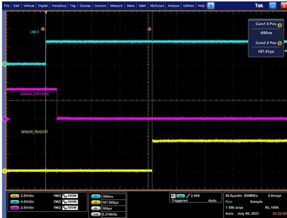
Figure 31: Example of the 12bits sensor data output delay, here 187.00 \mu s
