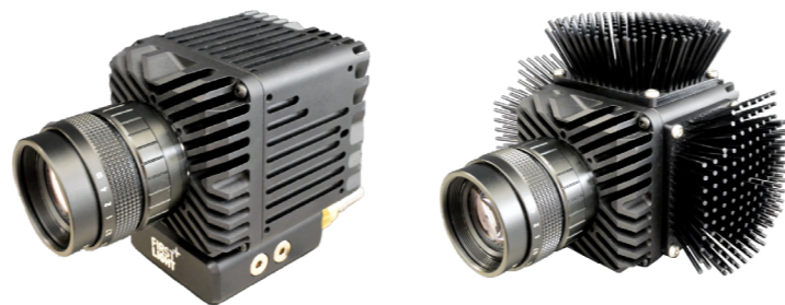
Hydraulic cooling plate (left) and passive heat sinks (right).
