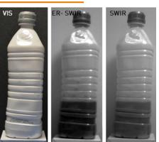
Visible versus SWIR and ER-SWIR images of a plastic bottle filled with water. The bottle is opaque in the visible range, while ER-SWIR increases the contrast compared to SWIR. Courtesy of First Light Imaging.
