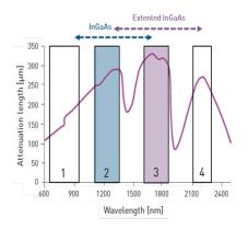
Transmittance in brain tissue of 200 µm thicknesses. Four spectral regions are identified. The third wavelength region can be exclusively detected by extended range cameras.
