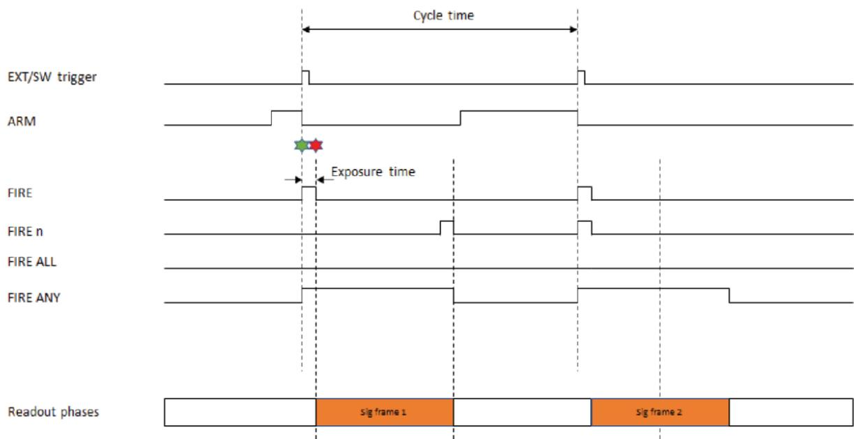
Figure 16: External Triggering “short” (non-overlap)
