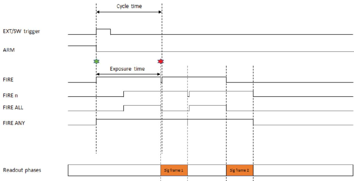
Figure 20: Rolling Shutter External Start Triggering (Non Overlap)
