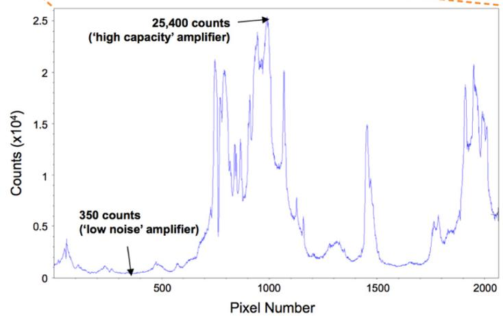
**Figure 9: High contrast image of fixed labeled cell. Intensity line profile through single row demonstrates pixel regions that were sampled by high gain (low noise) and low gain (high capacity) amplifiers.**
