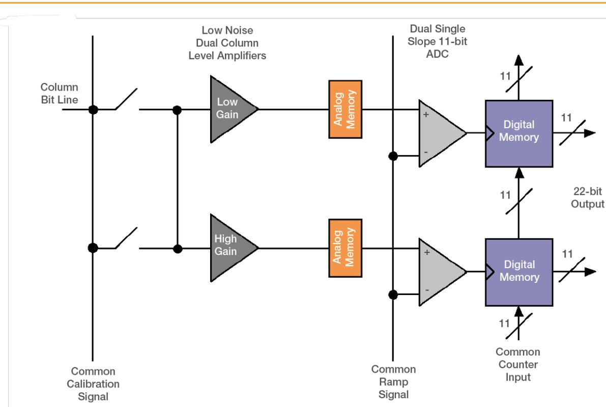
**Figure 8: Amplifiers and ADC of the sCMOS Sensor**
