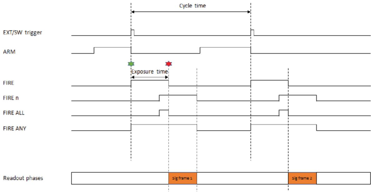
**Figure 17: External Triggering "long" (non-overlap)**
