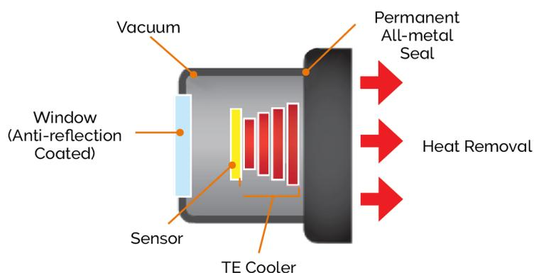
Outgassing is minimized through assembly in a state of the art facility, with a stringent protocol and use of proprietary materials (Outgassing is the release of trapped gasses that would otherwise degrade cooling performance and potentially cause sensor failure). UltraVac also features a single camera window for the best optical performance. For more information about our UltraVac technology, please visit our website and view the technical article on [UltraVac](#).
