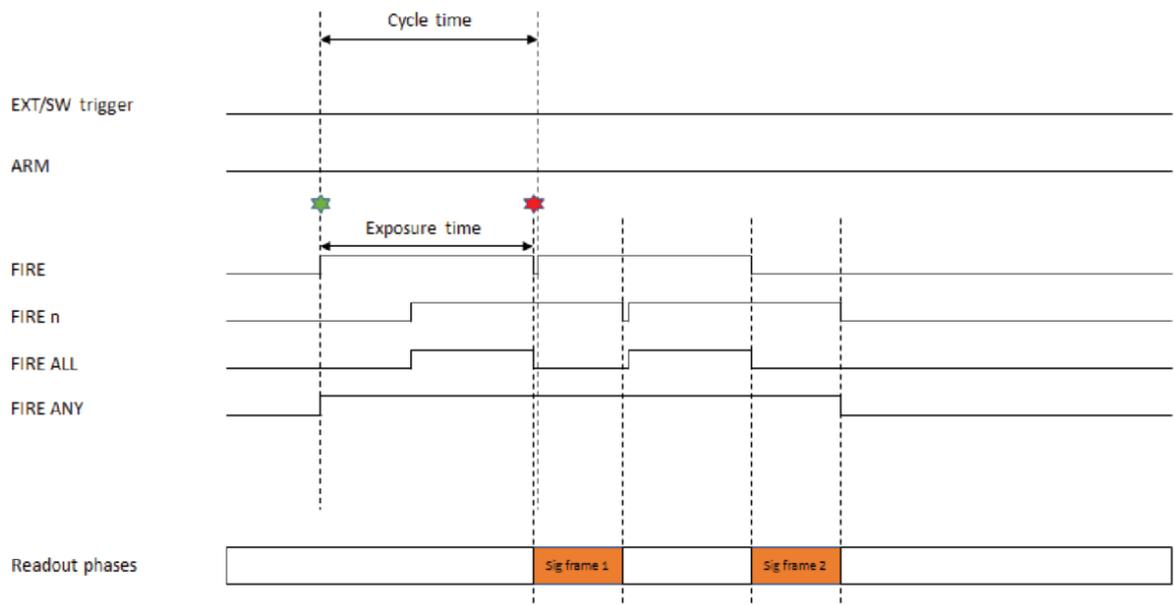
**Figure 15: Internal Triggering "long" (overlap)**
