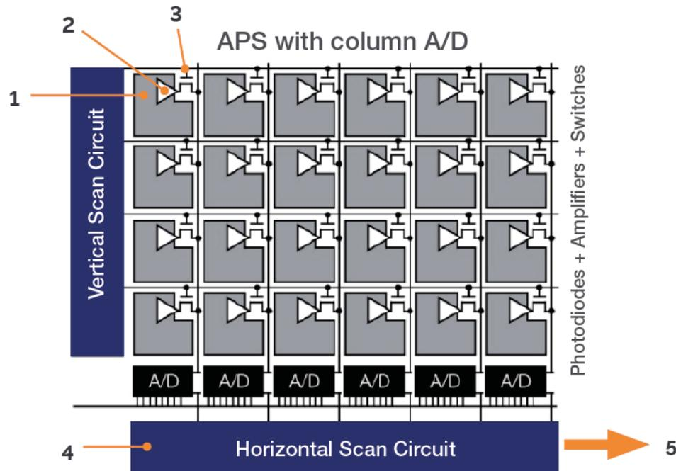
As illustrated above, the CMOS sensor is an “Active Pixel Sensor” (APS) whereby each pixel has its own integral amplifier and the sequence of operation is as follows:
