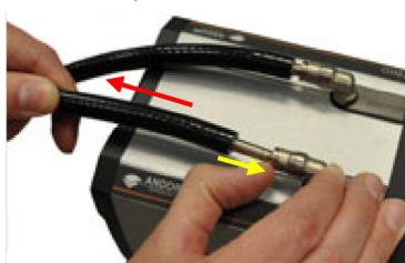
FIGURE 45: PRESSING THE LATCH ON THE CONNECTION TO RELEASE THE COOLANT HOSE
