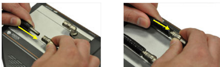
FIGURE 43: CONNECTING THE HOSE FITTINGS TO THE CAMERA COOLANT CONNECTORS
