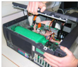
FIGURE 38: REMOVING THE COMPUTER COVER
