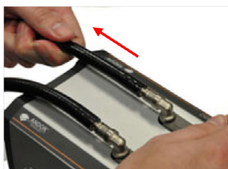
FIGURE 44: TESTING COOLANT HOSES ARE SECURELY CONNECTED
