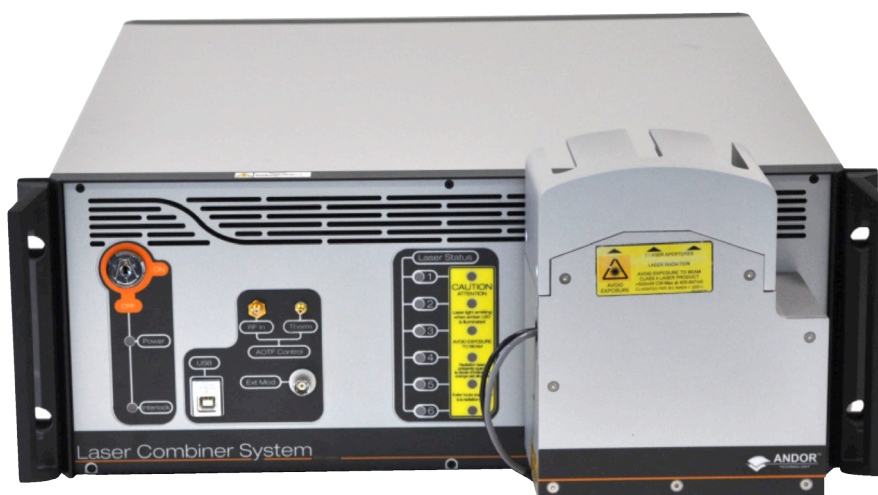
Figure 3: The Multi-port Unit (MPU) Head attached to an ALC601.
