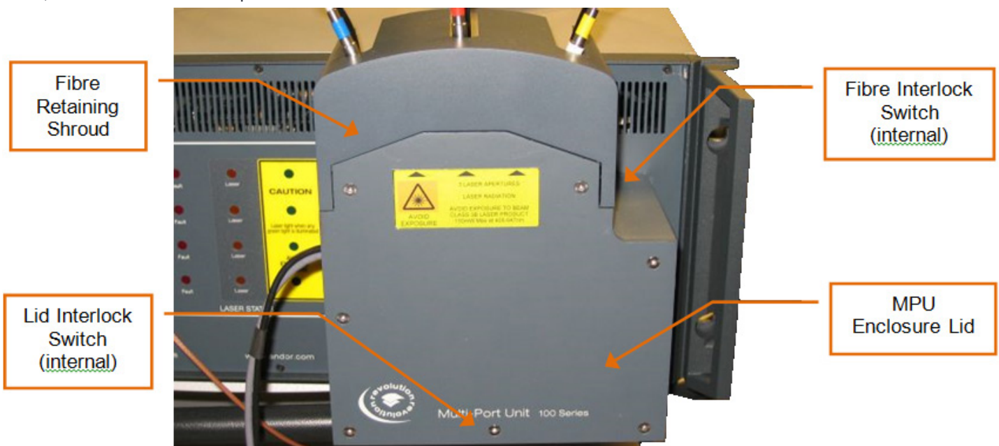
Figure 13: MPU Head and Interlock Features (note that this shows an image of an early production unit).
