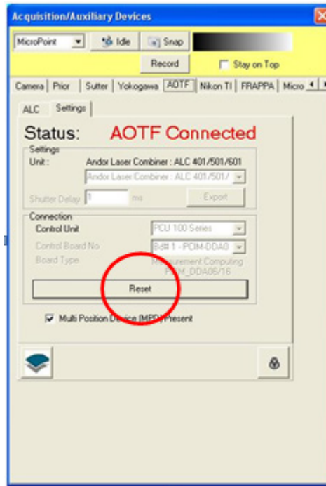
Figure 15: Resetting the Interlock System after Closure of Interlock Switches
