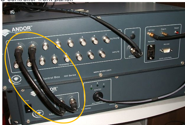
Figure 11: MPU to PCU Connection
