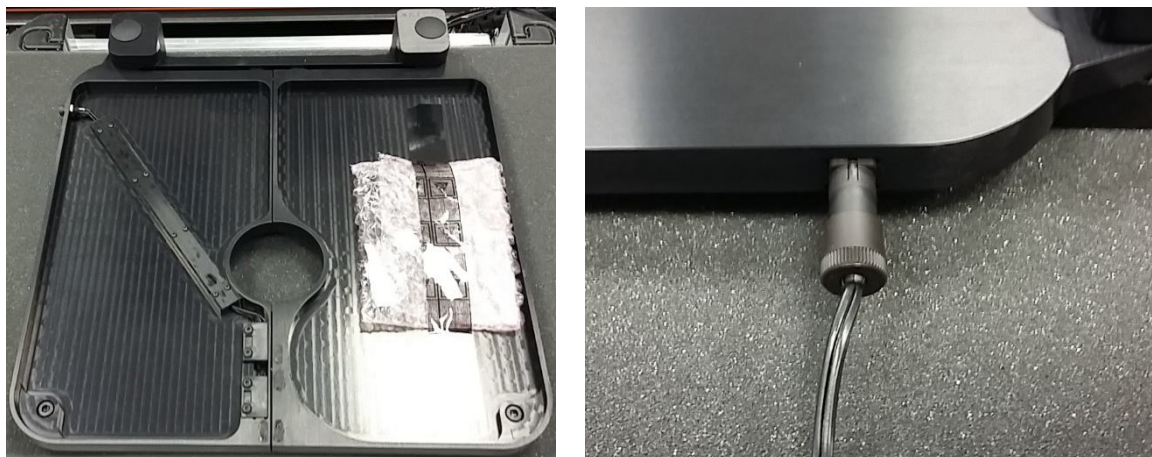
Figure 3: External Interlock Cable (ASE-11399) in Bag Underneath Stage Cover and Connected
