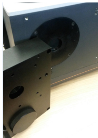
Figure 8: Removal of the filter wheel (left), once removed the shutter can be accessed (right).
