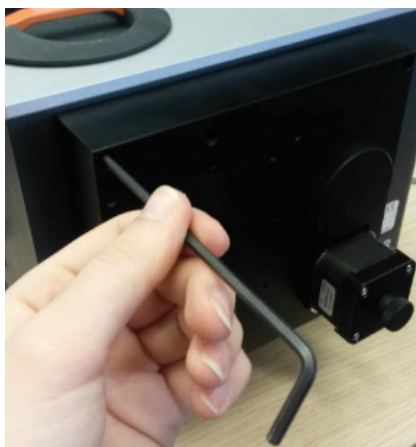
Figure 8: Removal of the filter wheel (left), once removed the shutter can be accessed (right).
