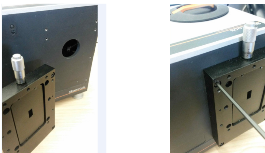
Figure 9: A range of slits can be installed as required.
