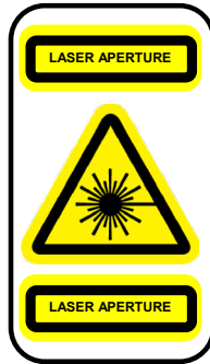
Figure 2: Laser aperture warning label on BCU optical fibre output
