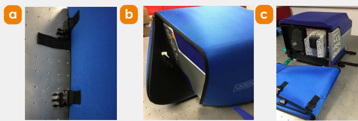
Remove the dust jacket on the BC43 unit. a) Unclip the side straps. b) Unzip the side panel. c) Remove the dust jacket.
