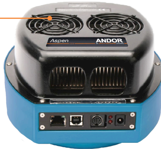
Figure 2: View of Aspen showing Cooling fans
