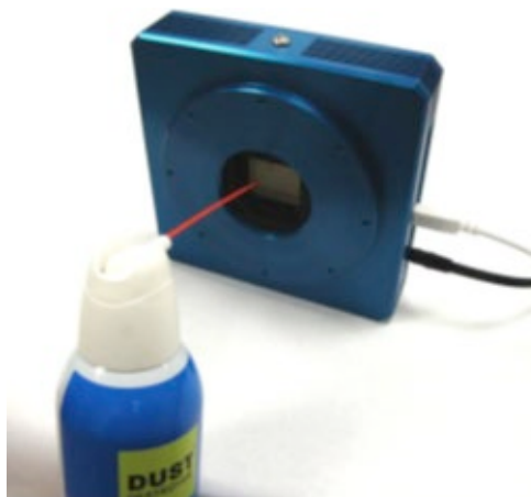
Figure 7: Using Compressed Air to remove dust from the camera window
