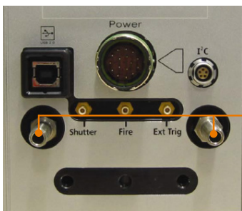
Coolant hose connectors for connection to the cooling system
