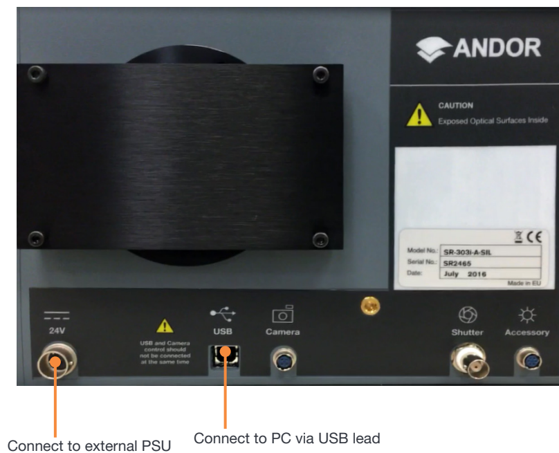
Figure 3: Connecting the power and USB cables to the spectrograph
