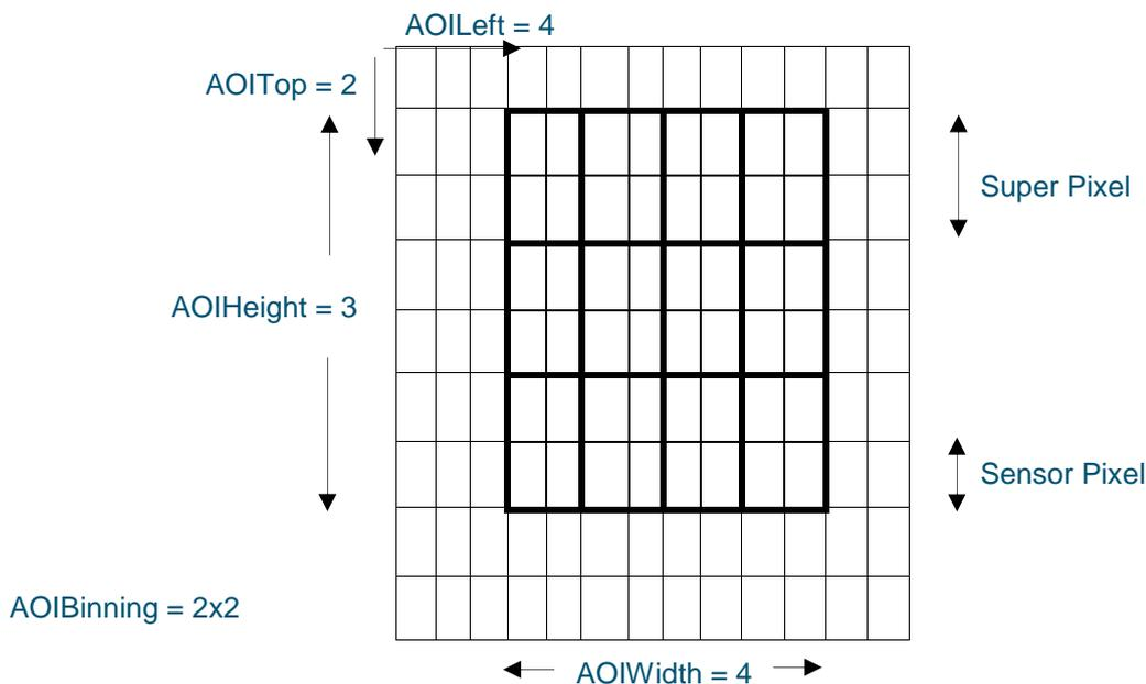
**Figure 4: Configuring an AOI and presentation of Super-Pixels**
