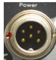
**Power:** connection for the **Power Supply Block (PSB)** shown on the next page.
