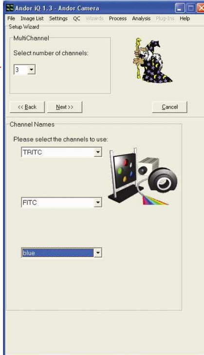
**NOTE:** Again, channels remain non-frame transfer. You do not need frame transfer operation when you have to change filters between exposures.
