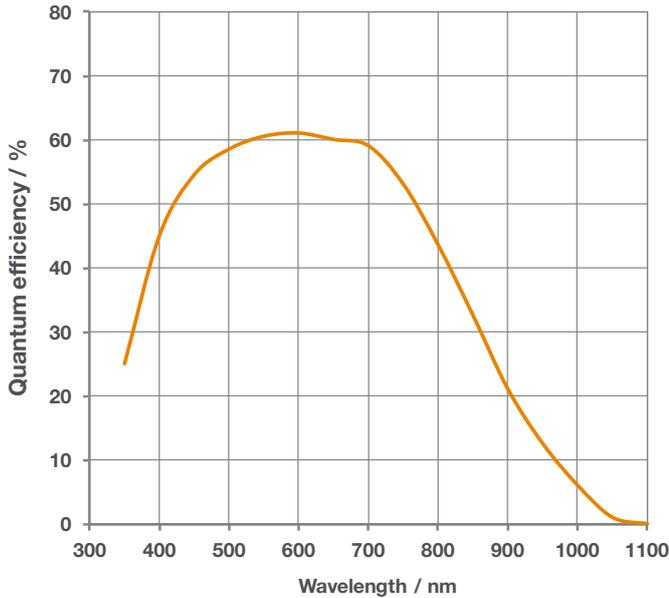
**Balor 17F-12 does not suffer etaloning effects across the important NIR wavelength range, preserving accurate photometry and spectroscopy**
