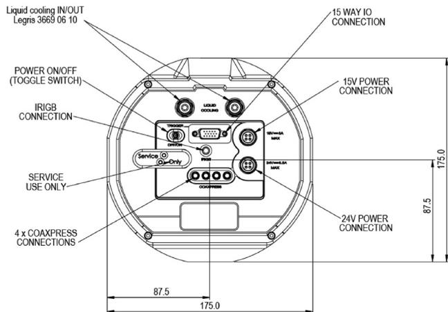
Note: air vents are not present in the housing of the Liquid Cooled Only model (not shown). This option can be selected for minimal thermal bloom.
