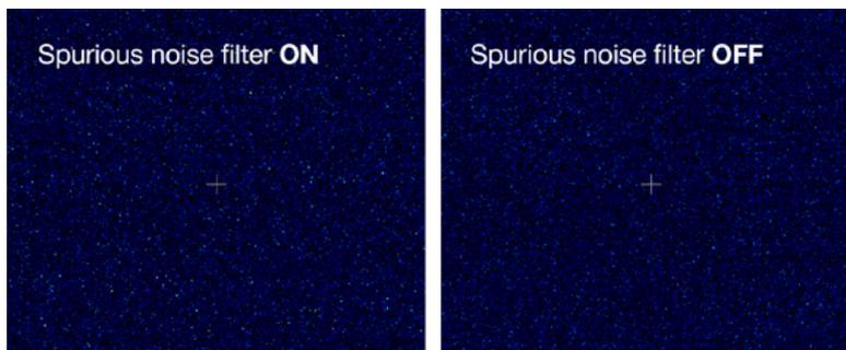
Figure 8: A demonstration of the effect of the Spurious Noise Filter, on a dark image, 20 ms exposure time.
