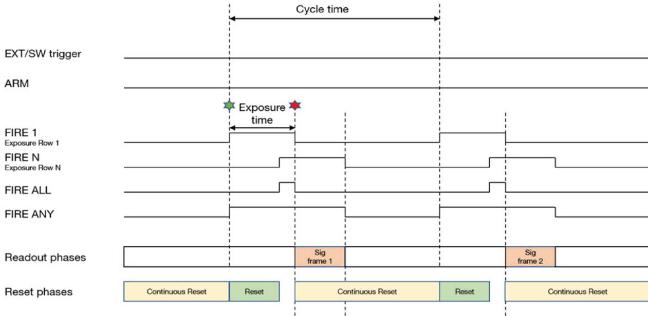
Figure 12: Rolling Shutter Internal Triggering (Part 2: exposure time > readout time).
