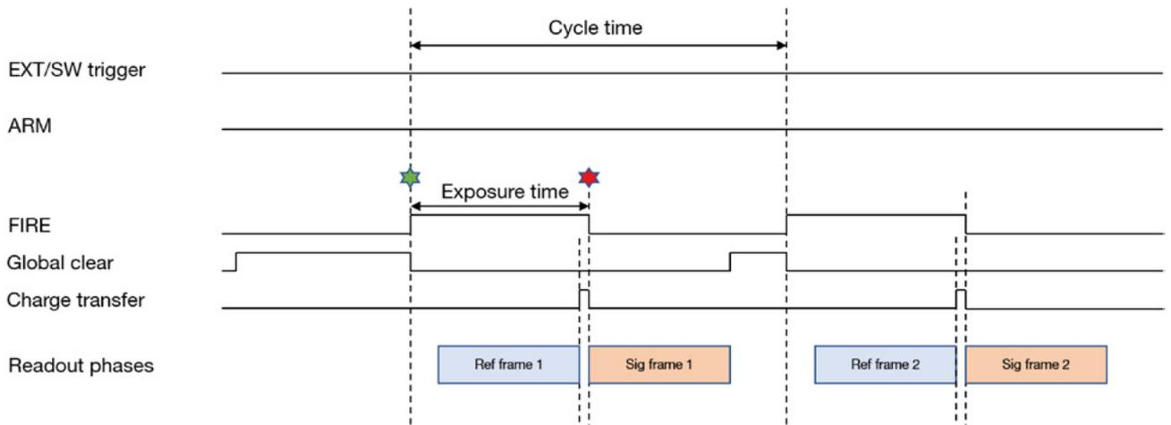
Figure 21: Global Shutter Internal Triggering – Long Exposures.
