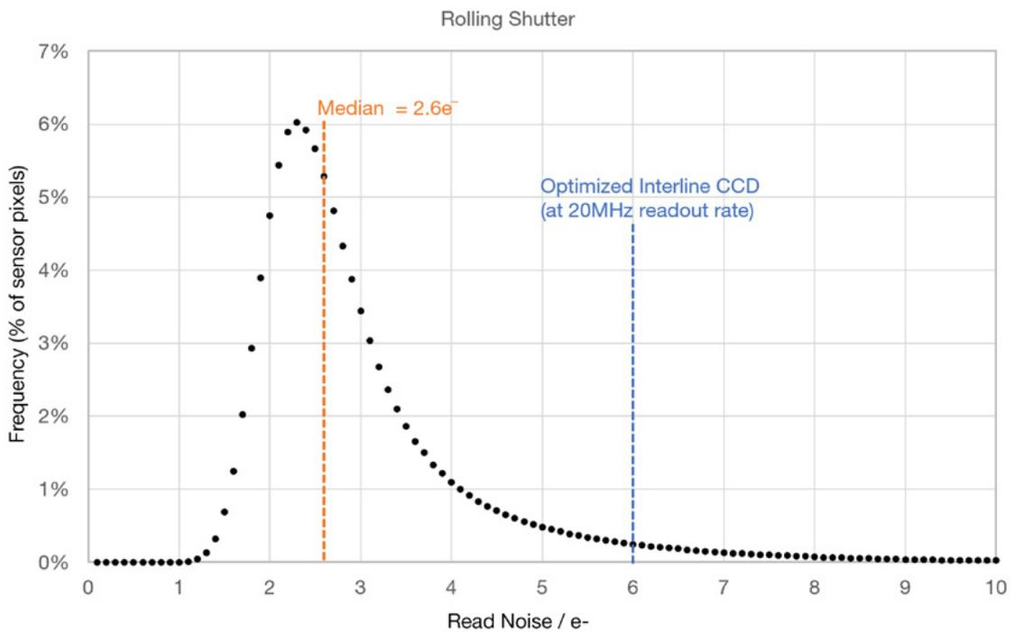
Figure 7: Representative histogram showing read noise distribution at fastest readout speed of the Balor. The line at 6 e- represents a typical read noise value from a well optimized Interline CCD – all pixels in a CCD essentially share the same noise value.
