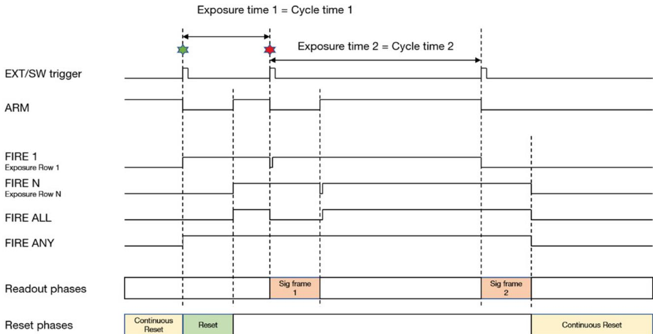
Figure 18: Rolling Shutter - 100% Duty Cycle - External Exposure.
