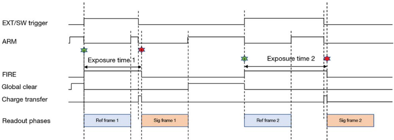
Figure 25: Global Shutter External Exposure Triggering.
