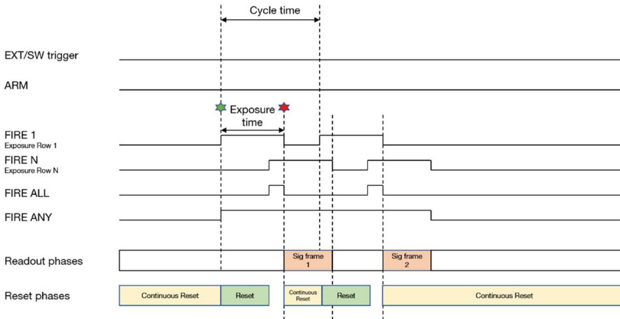
Figure 13: Rolling Shutter Internal Triggering (Part 3: Row 1, of the second exposure starts before, Row N, of the first exposure completes).
