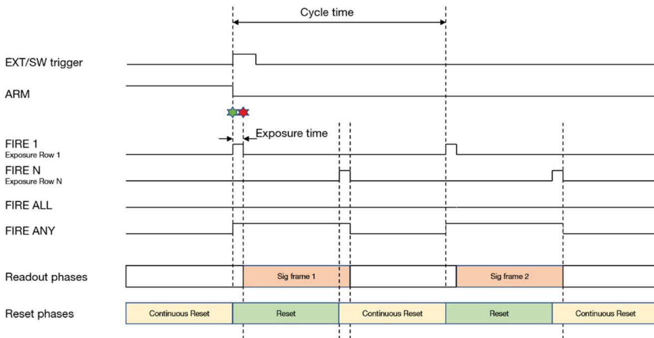
Figure 19: Rolling Shutter - External Start Triggering.
