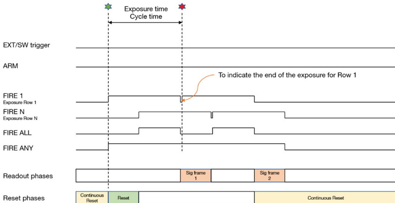
Figure 14: Rolling Shutter - 100% Duty Cycle - Internal Triggering.
