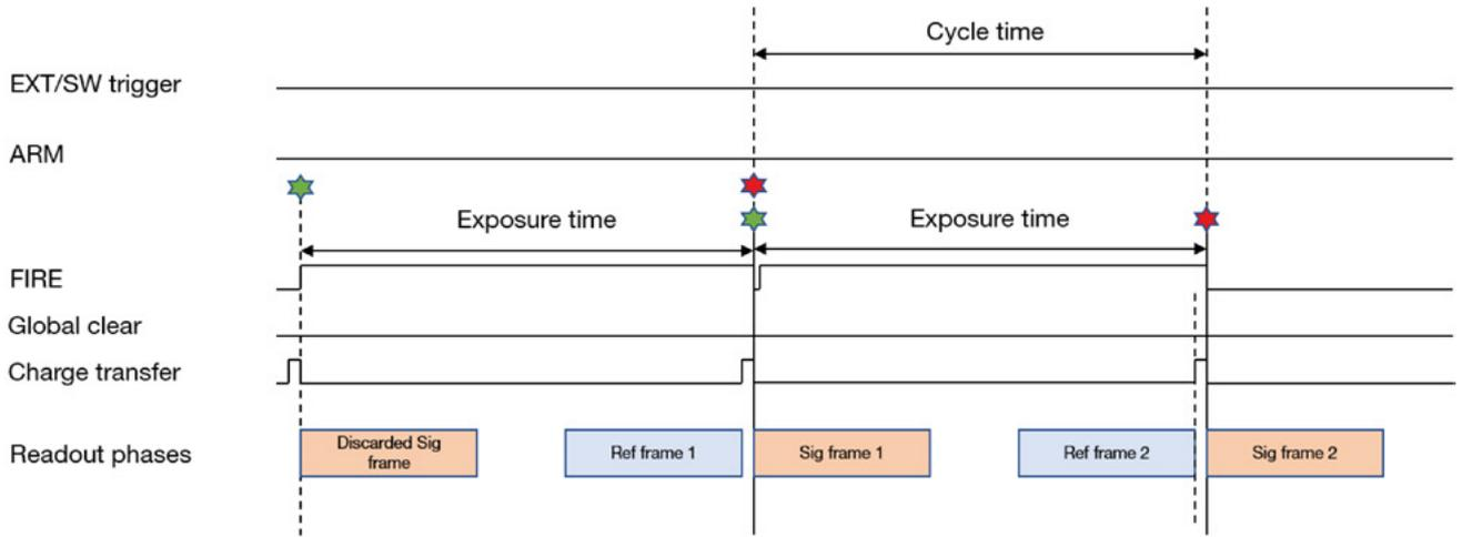
Figure 22: Global Shutter - 100% Duty Cycle Internal Triggering.
