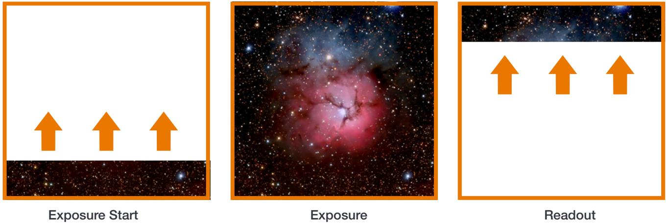
Figure 5: An illustration of Rolling Shutter sensor exposure.
