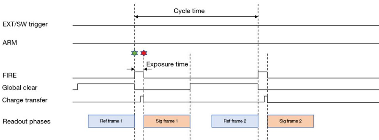
Figure 20: Global Shutter Internal Triggering – Short Exposures.
