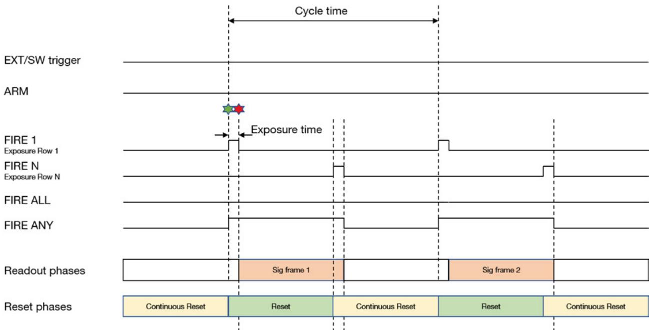
Figure 11: Rolling Shutter Internal Triggering (Part 1: exposure time < readout time).
