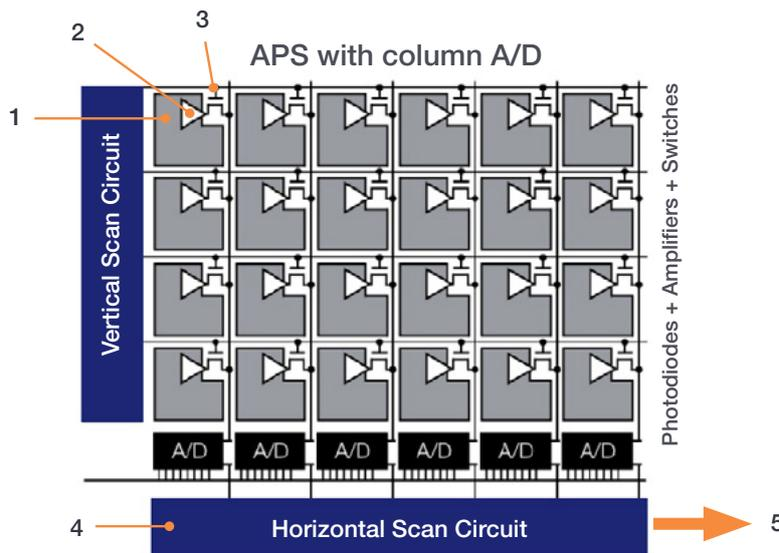
Figure 4: sCMOS sensor architecture.
