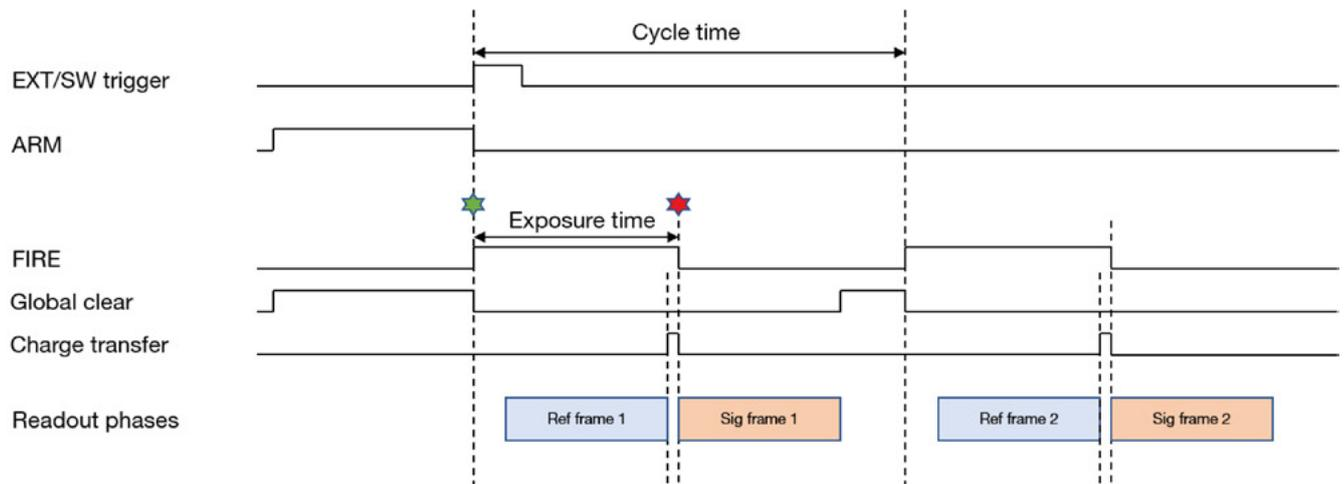
Figure 24: Global Shutter External/Software Triggering Long Exposure.
