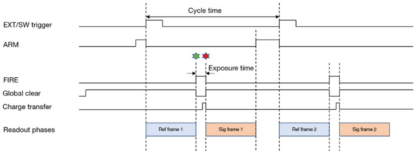
Figure 23: Global Shutter External/Software Triggering Short Exposure.
