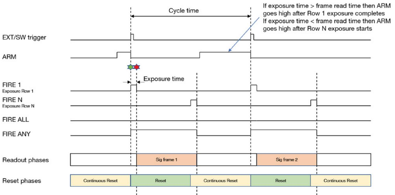
Figure 15: Rolling Shutter - External Triggering (Part 1: exposures separated).
