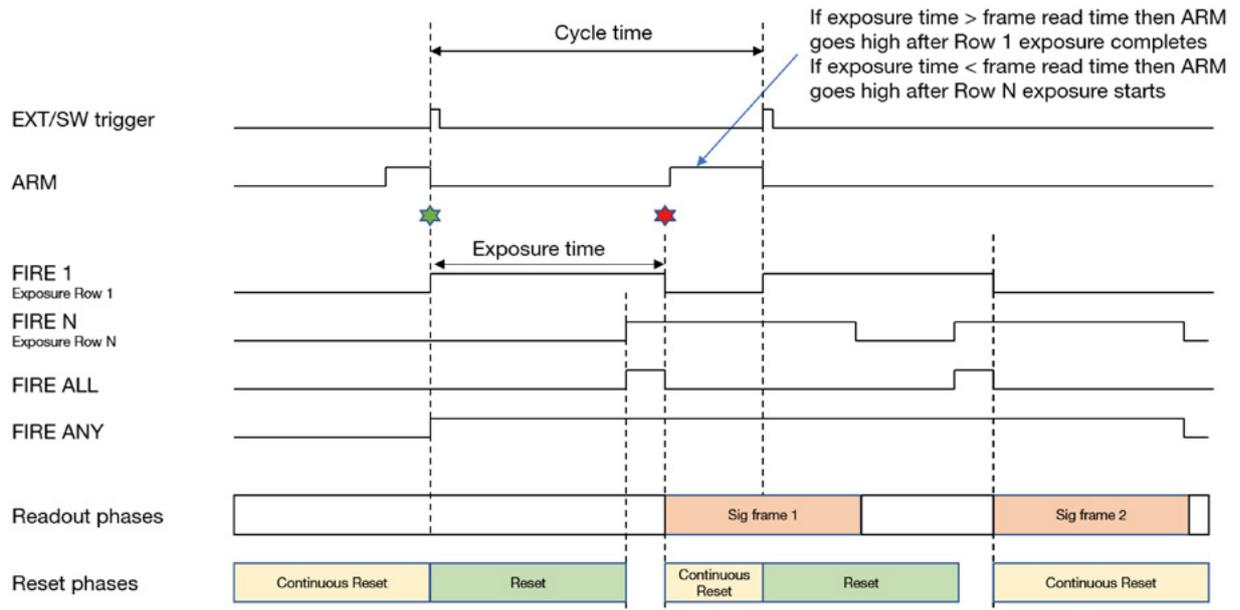
Figure 16: Rolling Shutter - External Triggering (Part 2: Second exposure starts before readout completes).
