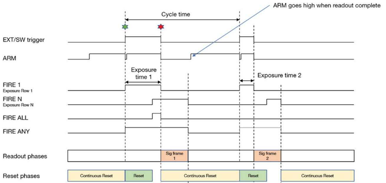
Figure 17: Rolling Shutter - External Exposure (Note exposure time can vary during series).
