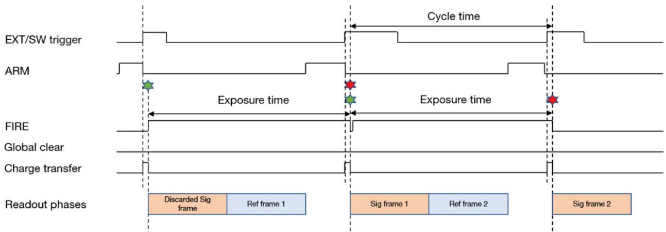
Figure 26: Global Shutter - 100% Duty Cycle External Exposure Triggering.
