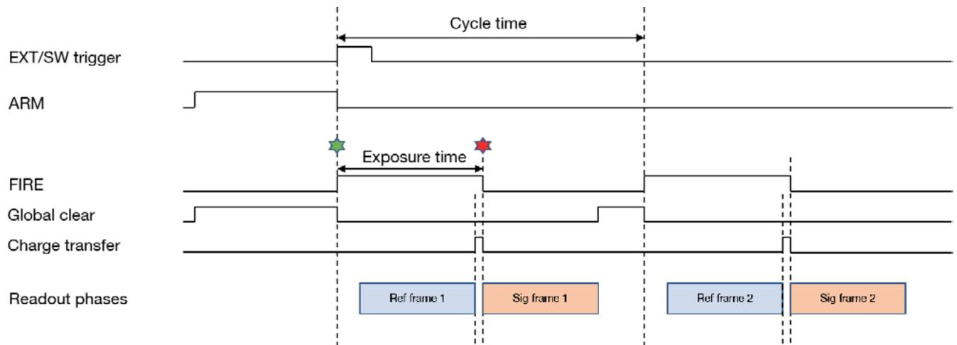
Figure 27: Global Shutter External Start Triggering.
