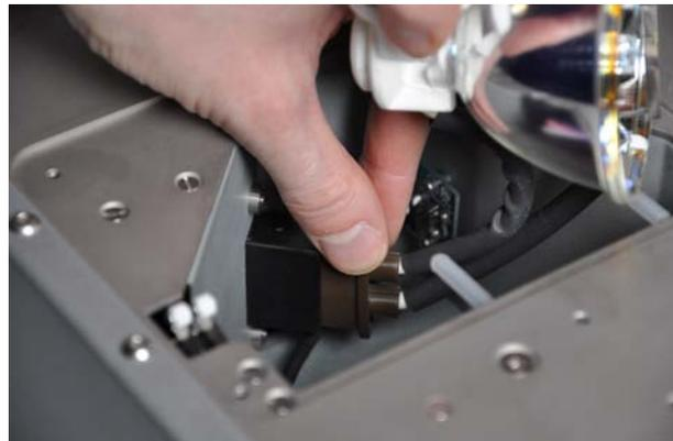
9. Locate the bottom of the lamp, as shown below and fit it into the lamp socket locating groove:
