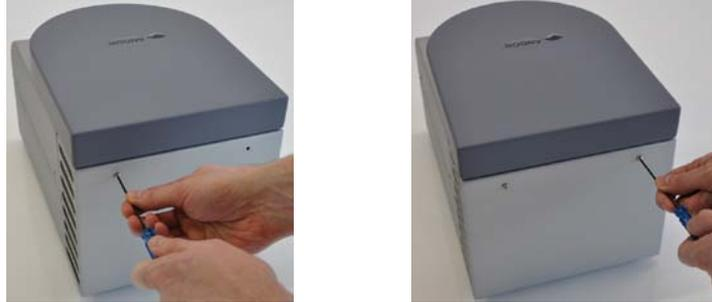
2. Turn the unit upside down and remove the remaining screw :
