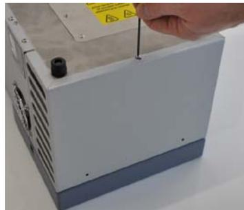
3. Turn the unit onto its feet and pull the rear cover away from the main body of the unit:
