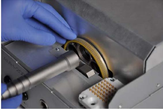
7. Filter rings are keyed to allow easy removal with the supplied filter ring access tool. To unscrew the filter ring, locate the keys into the matching slots of the filter ring and turn it anti-clockwise. When you have removed the filter ring, you can then proceed to remove any filter already in the recess:
