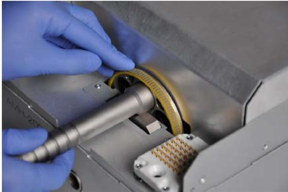
8. Place the new filter in the recess and secure it in position using the filter ring. Take care not to over tighten the filter ring as some filters will expand as they are heated by the light
