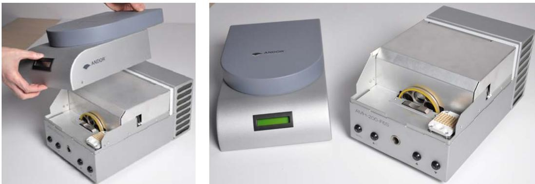
6. Turn the filter wheel by hand until the desired filter position is in the filter change position (the filter number is displayed on the top left of the filter hole):
