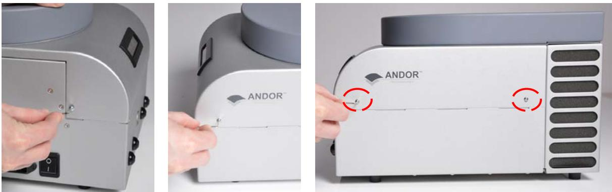
5. Lift the top of the unit then place it carefully to one side:
