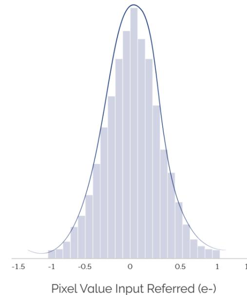
OCAM<sup>2</sup>S Noise Histogram for gain (x1000)
