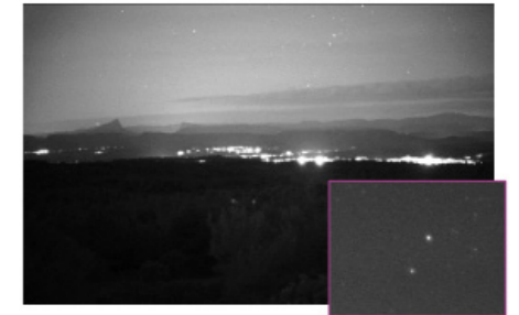
Detection of stars on a moonless night. Camera: Andor CB1 1.7 MP. Objective lens: 35 mm f/1.4.
