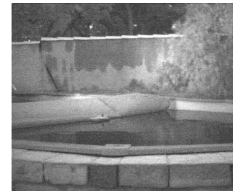
Night vision in the SWIR range. Imaging of a boat in a swimming pool, by a moonless night. Camera used: C-RED 2 with SWIR lens 16 mm, cooled down to -15^{\circ}\text{C} . High gain.
