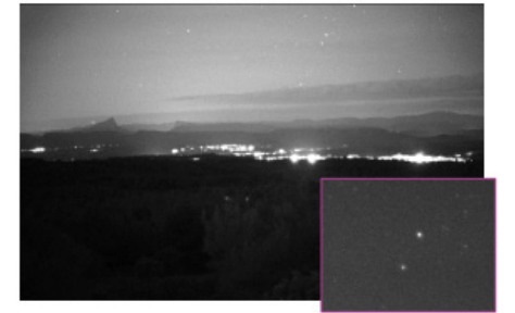
Detection of stars on a moonless night. Camera: C-BLUE One 1.7 MP. Objective lens: 35 mm f/1.4.
