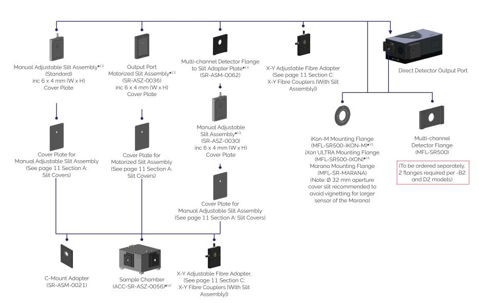
Note: a flange MUST be ordered separately for any configuration involving a multichannel or InGaAs detector.
