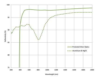
The graph shows the standard Al + MgF<sub>2</sub> optics coatings reflection efficiency versus wavelength.
