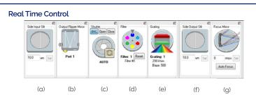
(a and f) Slit drive: Control the spectrograph slit width - drag blades on icon or type in required slit width
